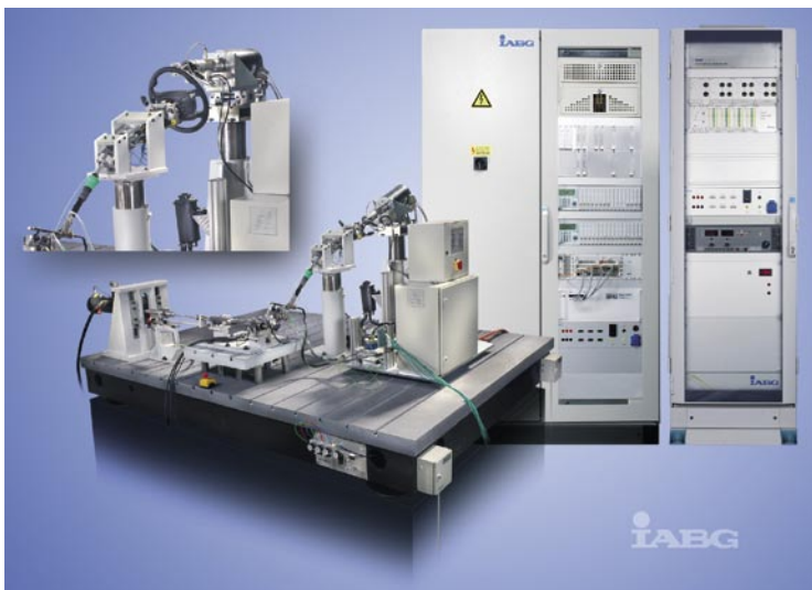
▲ The HIL test bench has proved to be an effective tool for testing active steering.
